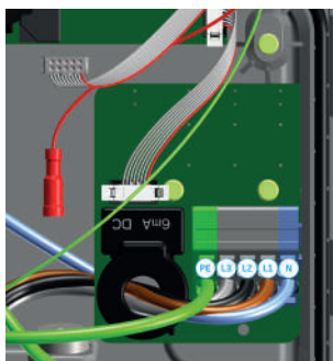
Figure 8b: Connection clamps power and Control Pilot (CP) connector for the charging cable (red) to S-line 3 phase, Pro-line.
